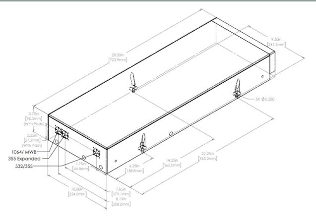
Photonics Industries RX Series picosecond lasers are all-inone (AIO) and do not require a separate controller or utility module. All connections for operation and control of the laser can be found on the back panel of the AIO laser.
